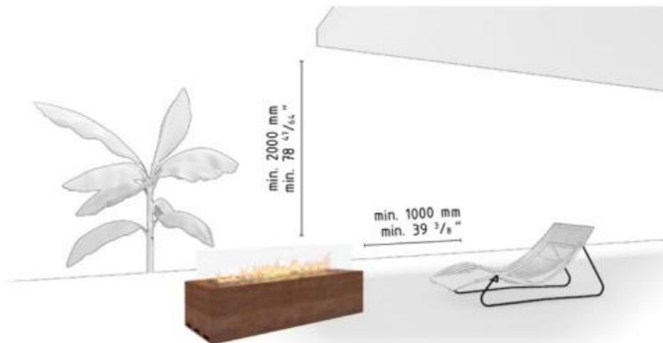
Fig. 1: Minimum distance to flammable materials
