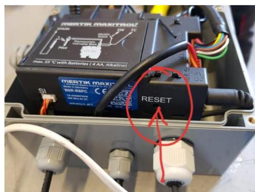
Fig. 7 – Receiver “RESET” button
